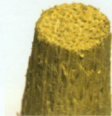
Close up of tip of a porous soft spile
